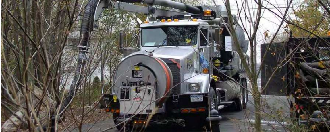
Figure 3-17: Sediment build-up in sumps should be removed using a vacuum or vector truck depending on the size of the system.
